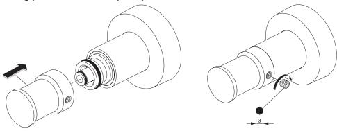
Push the caps onto the inlets until they stop against the shoulder. Take care not to damage the o-ring seals.
