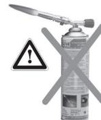
**DO NOT** apply heat near this product. Heat generated by soldering could damage plastic parts and seals.
