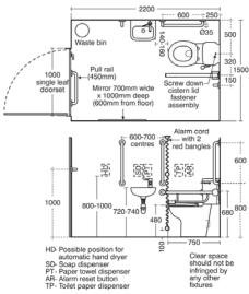
This layout is only suitable where it is not the only toilet facility within the building Wall and floor finishes must contrast visually
