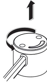
1. Twist the handle cap anticlockwise and lift it off
