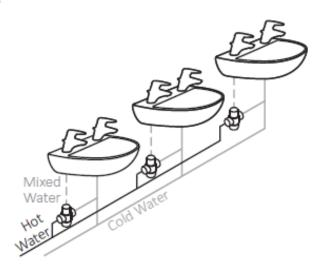
2 Consideration must be made for the possibility of multiple/simultaneous demands being made on the supply system whilst the A5900/1 AA valves (15 mm & 22 mm) are in use, all practical precautions must be made to ensure that the valve is not affected. Failure to make provision within the pipe sizing etc. will affect the performance of the valve.
