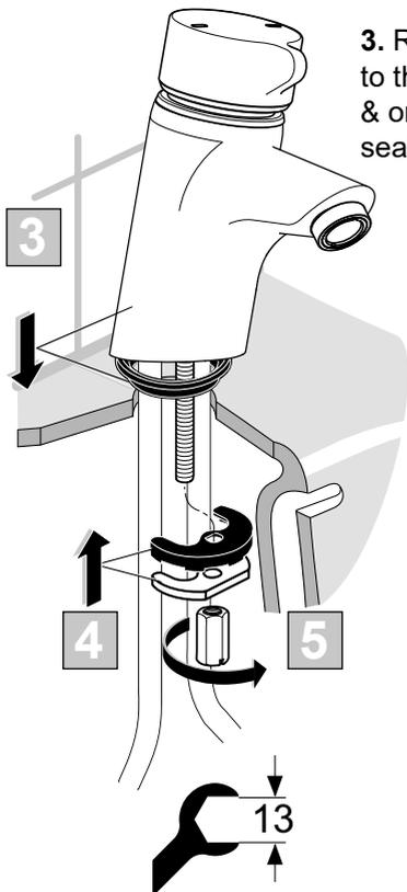
3. Remove the fixing kit parts if already assembled to the fixing stud. Ensure the basin seal is in place & orientated as shown. The larger diameter of the seal should locate into the base recess of the mixer. Offer the mixer towards the basin hole.
