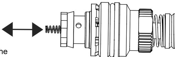
Before reassembling the cartridge cap, make sure that the filter screen is clean (slides out from inside of cap). When reassembling, take care to ensure the spring is straight & locates correctly into the boss at the bottom of the cap moulding.
