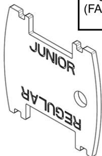
To change the outlet, use the outlet key supplied with the product to unscrew the AV housing. Using the side of the key marked "junior" locate the key into the inner ring of the housing and unscrew. Change the outlet & re-secure the housing with the key, ensuring the seal is in place.
