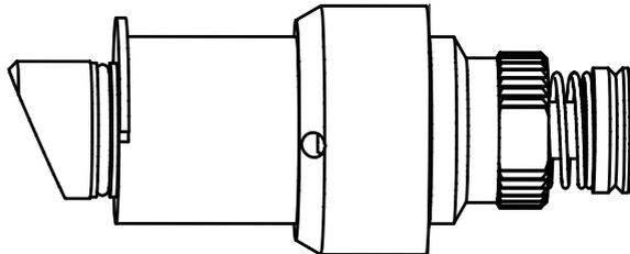
To access the cartridge assembly, first remove the brass housing shown. The lobe on the brass housing will prevent rotation when secured gently in a vice. Use 22mm spanner to unscrew the cartridge from the housing.
