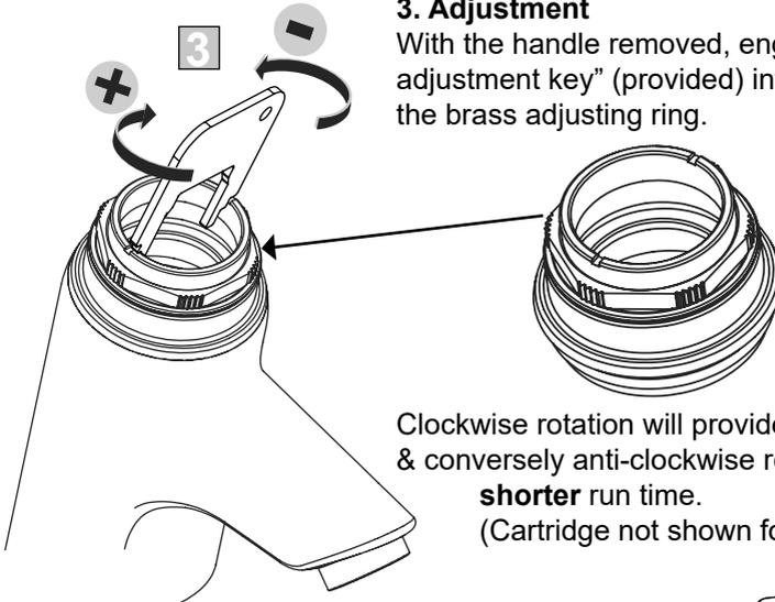
Clockwise rotation will provide **longer** run time, & conversely anti-clockwise rotation will provide **shorter** run time.
