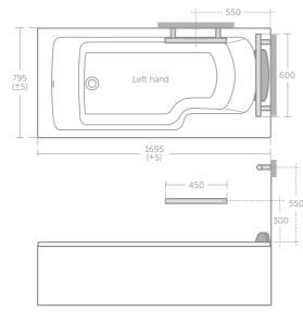
Positioning of the rails is advisory and should be positioned according to height and preference
