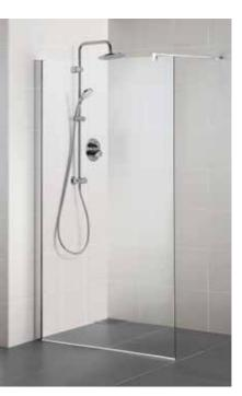
Height 2000mm 8mm clear safety glass Idealclean treatment 23mm horizontal adjustment Concealed fixings with easy click covers & top caps Sealing channels for a silicone free look Vertical adjustment for drilling into grout lines Suitable for installation on a tray or wetroom floor For full details of modesty panels see Concept Freedom.
